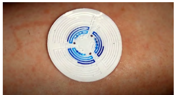
The “sweat sticker” collected 33% more sweat than the current test in a recent study.
